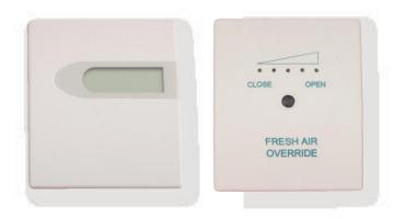
The SVC receives signals from the Temp/ $CO_2$  sensor and produces a 0-10v dc control output to modulate motorised ventilation units. The output is displayed on the LEDs on the fascia of the unit.
